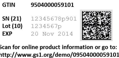
Figure 4.14.1-3. Combination of HRI with AIs, Non-HRI Text (GTIN and Expiry) and data titles
